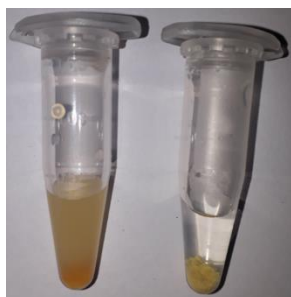
Figure 10: showing the adsorption (left vial) and desorption of metal ion (right vial) from the sensor.
