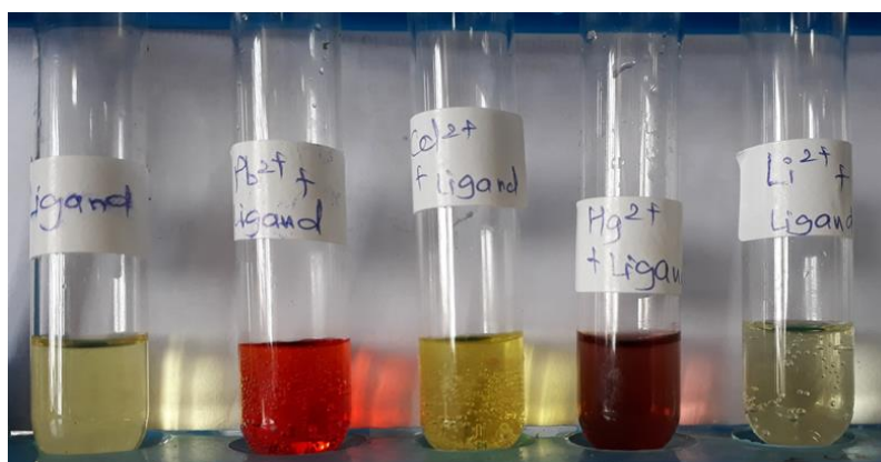
Figure 6: Screening of different metal ions for checking the response of sensor for other metal ions.
